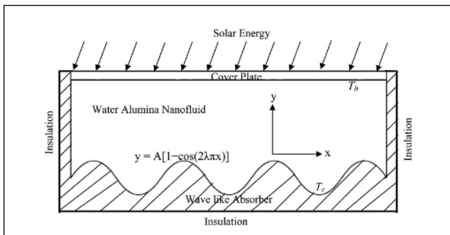
Fig. 2: Schematic view of a solar collector
