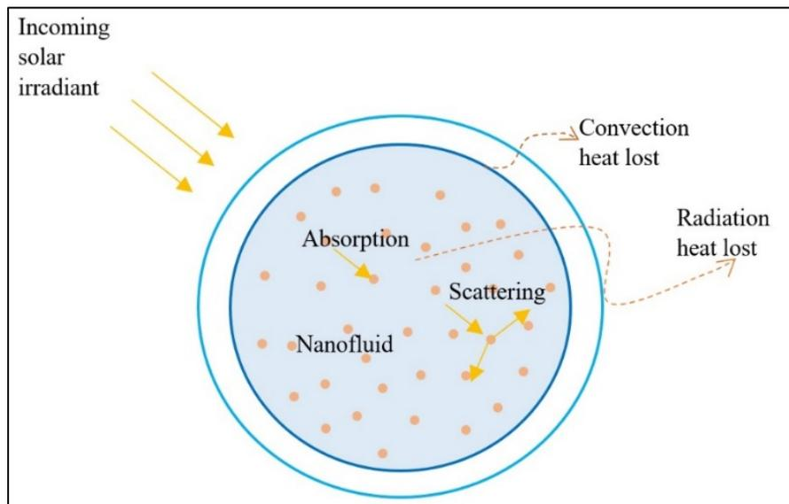
Fig. 1: Schematic view of the receiver of a solar collector
