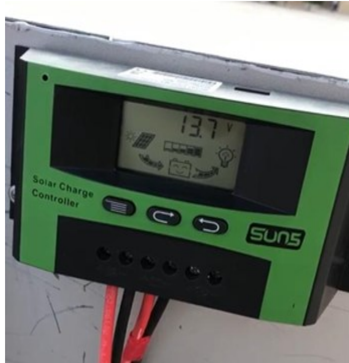
Figure 3.4: Charge controller output.
