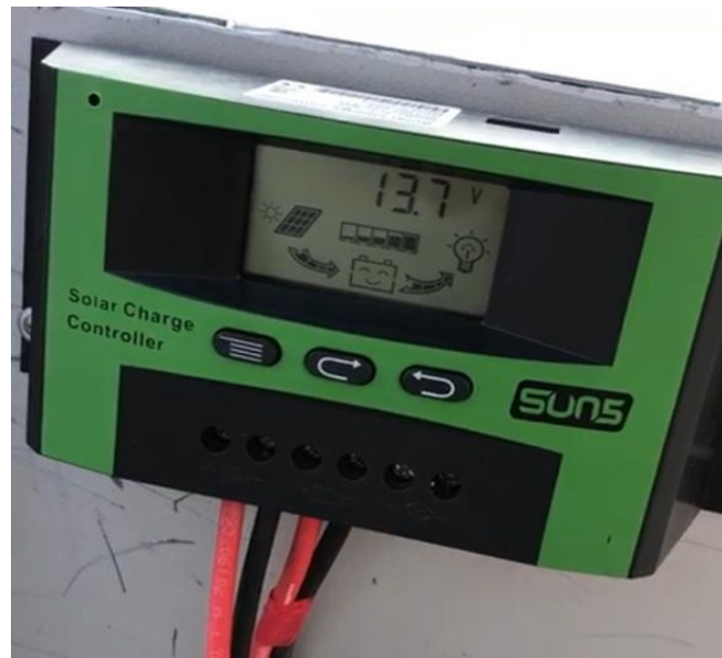
Figure 4.1: Charge controller output.
