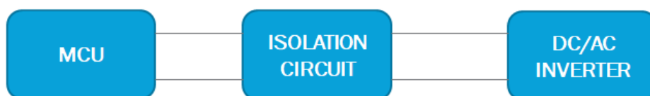
Figure 3.5: DC/AC inverter block diagram.
