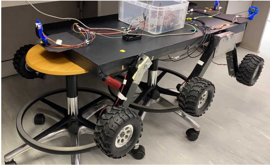
Figure 33: Temporary wheel installed in the rover.
