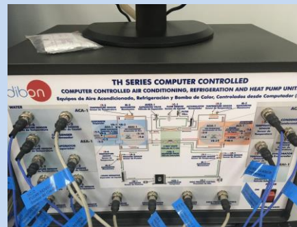
Figure 3 Computer Controlled Air Conditioning, Refrigeration and Heat Pump Units
