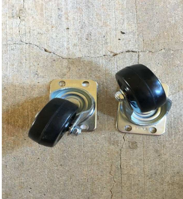
Figure Additional Supporting wheels used for dragging the Wheelchair when in folded position.
