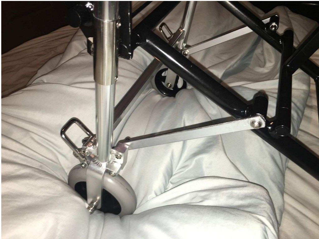
Figure The Assembled form of the Rear wheels support and their link to the Front Wheels Frame by the linking member and its Cylinder.
