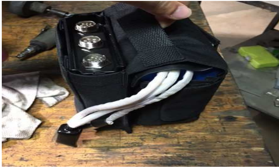
Figure Battery and controller bag
