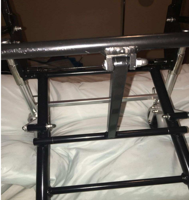
Figure The assembled form of the Seat Support and its connection to the Front Wheels Frame using the Rotation Cylinders.
