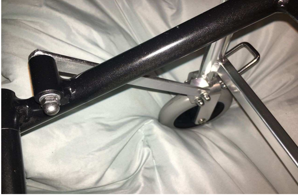
Figure The linking member between the Rear Wheel Support and the Front Wheels Frame.
