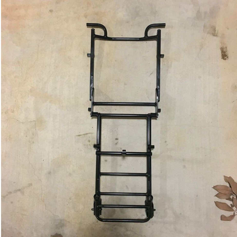
Figure Assembled form of the Front Wheels frame with the Back by means of the main Plate.
