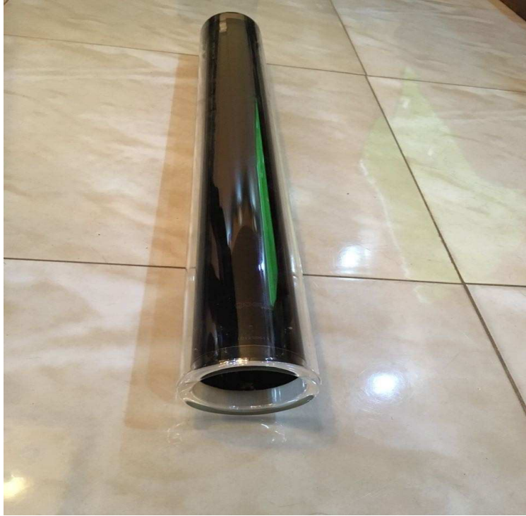
Figure 4.2: The Evacuated Tube
