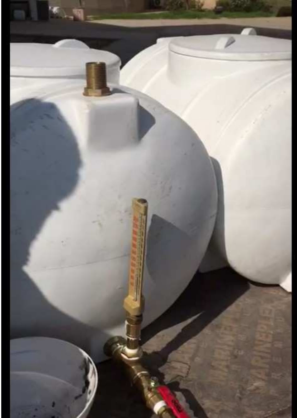
B.2 the inlet tank and the thermocouple that connected to the copper pipe
