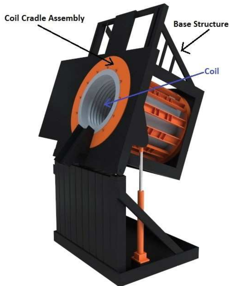
Figure .17 Induction Melting Furnace
