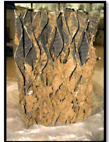
Figure.2.1 Scale deposits in the fill (Buecker, 2015)
