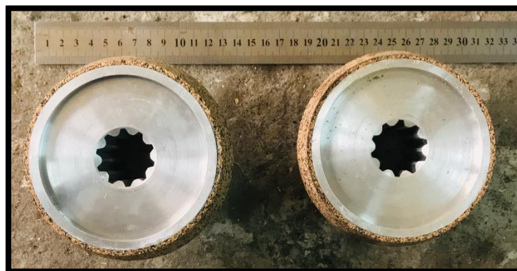
Figure # 3.4 (b): Machined Male Cones (Left: 12.5° & Right: 14.5°)
