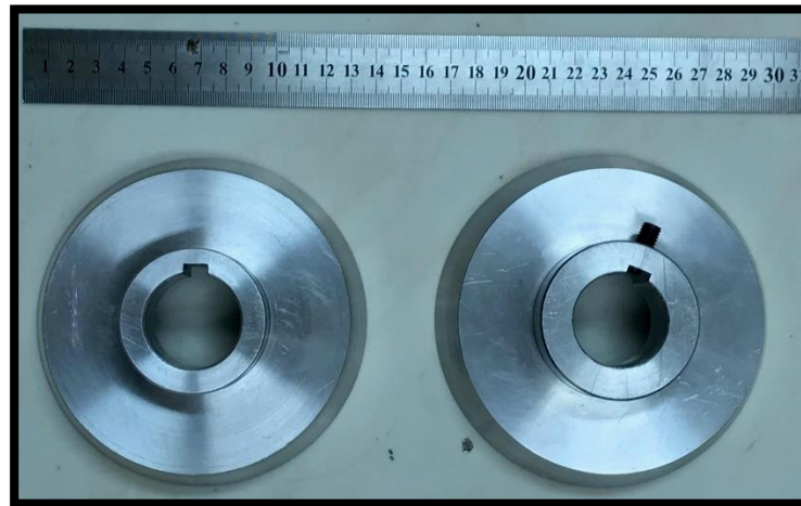
Figure # 3.4 (a): Machined Female Cones (Left: 14.5° & Right: 12.5°)
