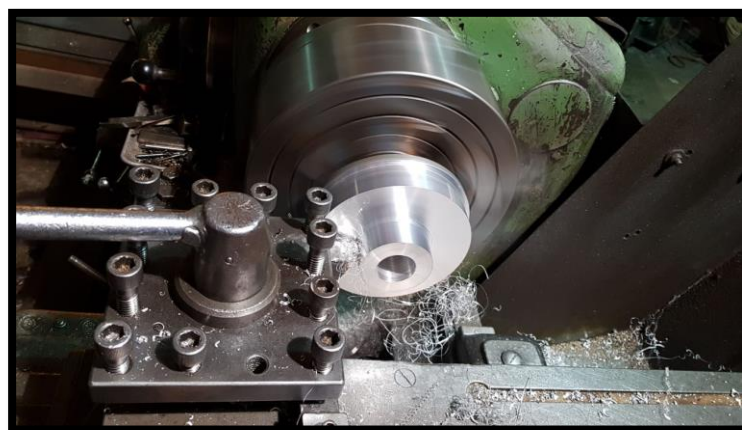
Figure # 3.5: Machining of Female Cone
