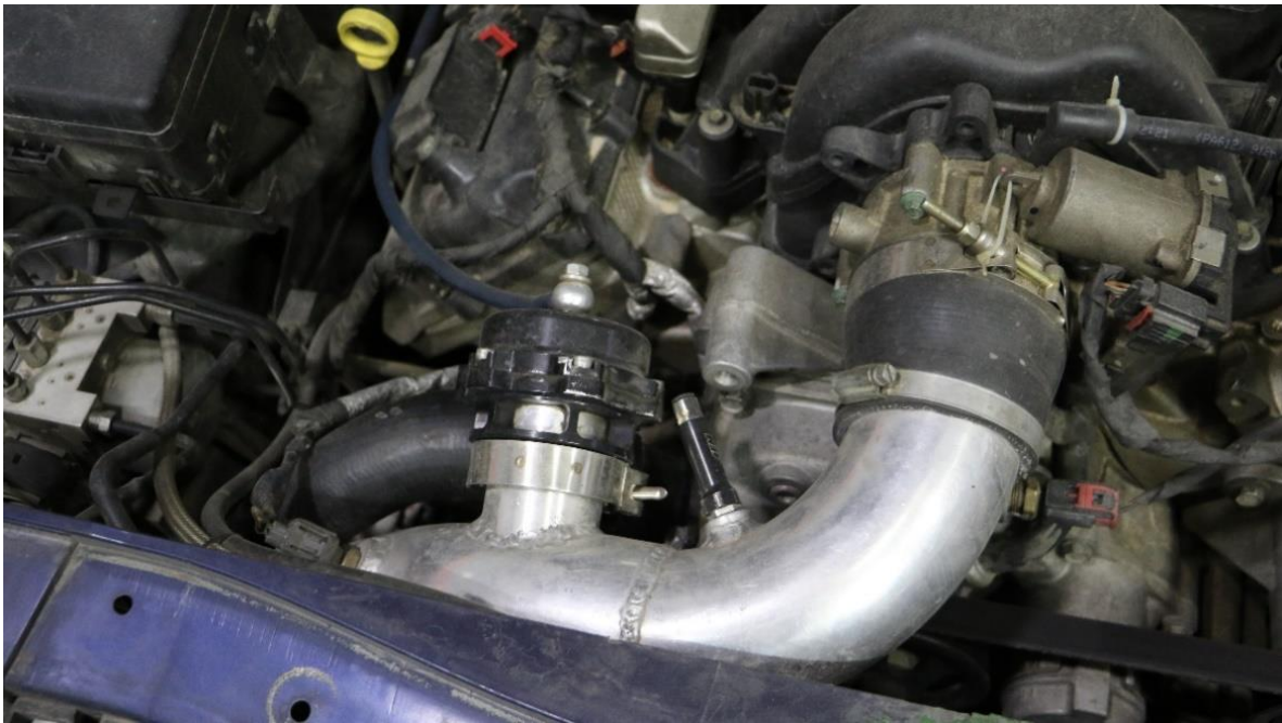
13Figure 3.10 Blow of valve
