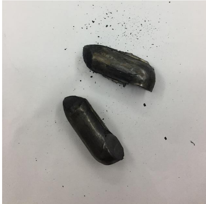
Figure 3.15: 4 passes Nanostructure Titanium 50 mm length, 22 mm Diameter
