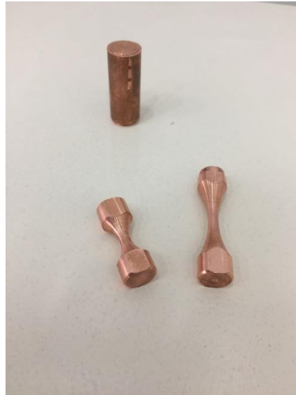
Figure 3.11: Two Specimen with 53.23 mm and 36 mm length for torsion test
