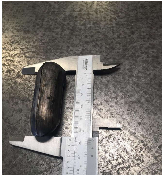
Figure 3.14: 2 passes Nanostructure Titanium with scale
