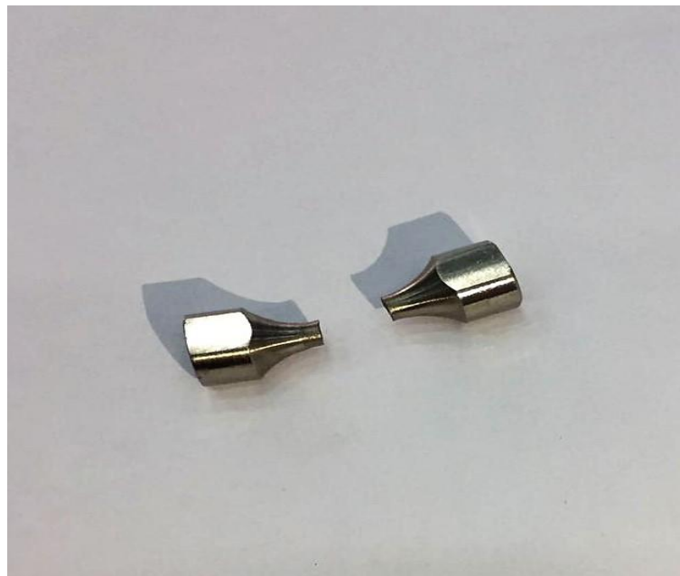
Figure 3.7: The specimen after the Torsion Test.
