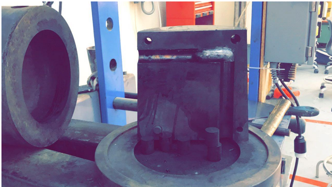
Figure 3.9 Die ECAP Process after one pass
