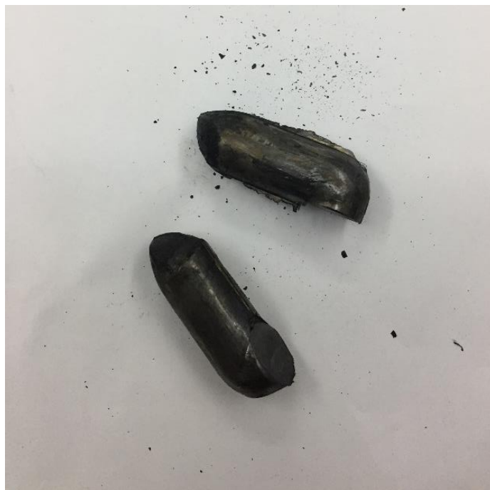
Figure 3.15: 4 passes Nanostructure Titanium 50 mm length, 22 mm Diameter
