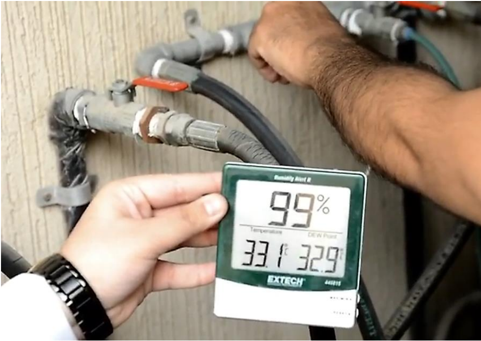
Figure 4.2 (Shows the humidity result before connecting the supersonic nozzle separator system)
