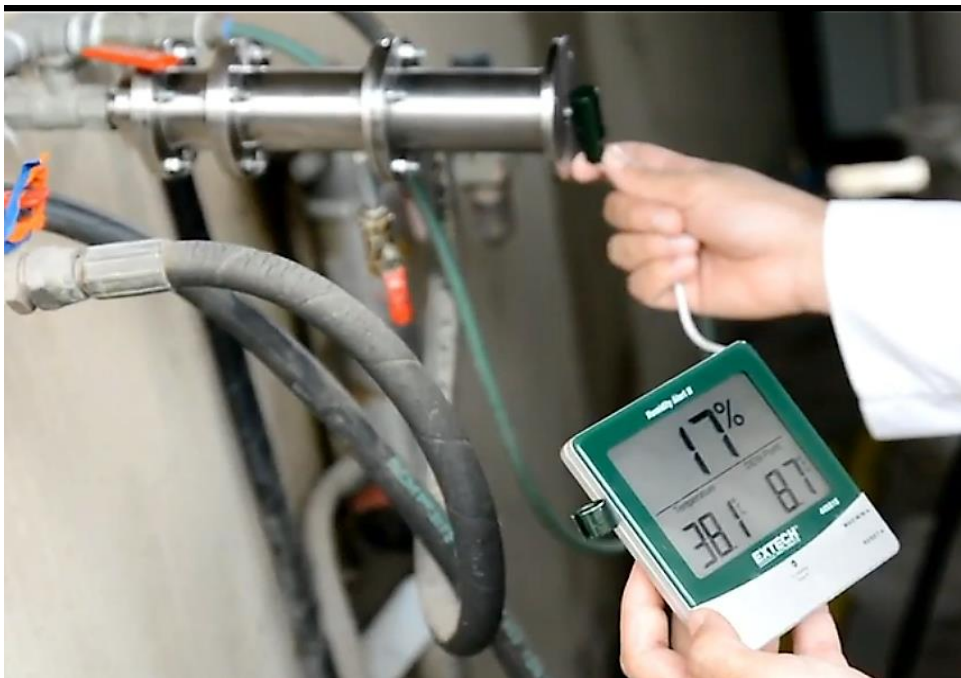
Figure 4.5 (Shows the humidity result of the supersonic nozzle separator system with 90mm diffuser)
