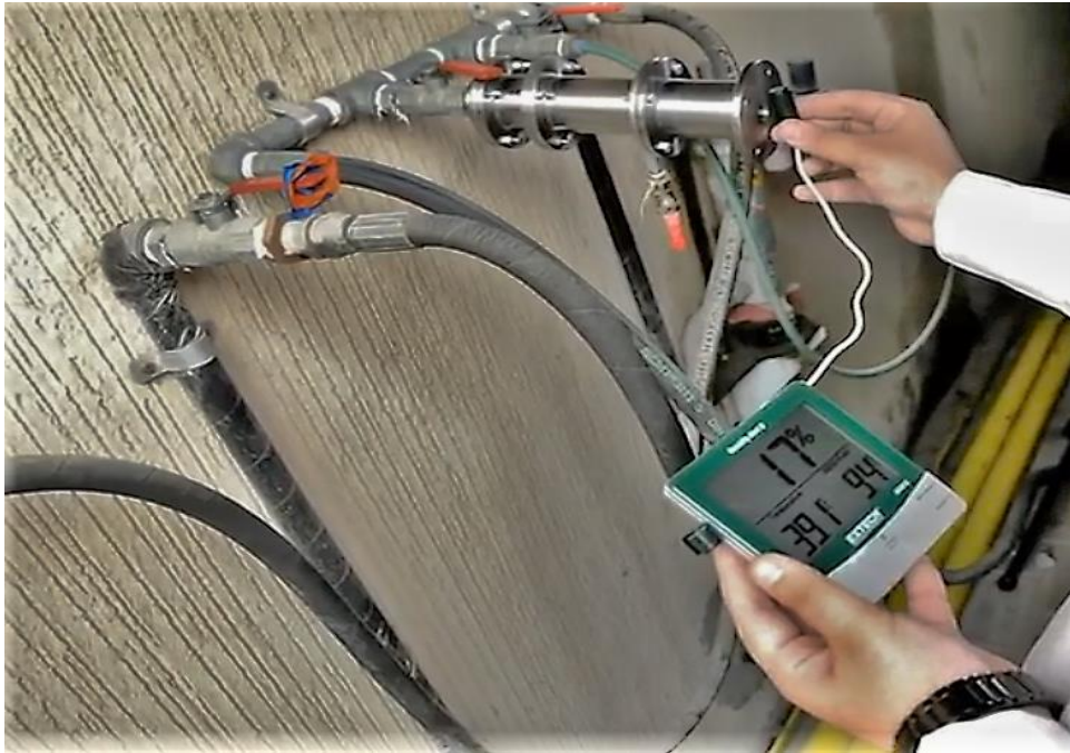
Figure 4.4 (Shows the humidity result of the supersonic nozzle separator system with 70mm diffuser)
