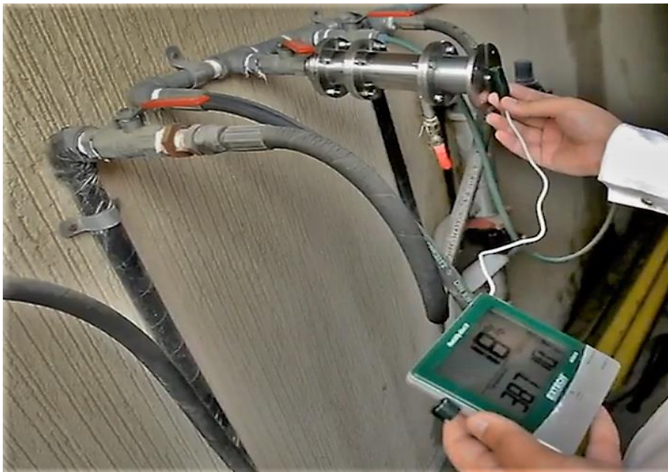
Figure 4.3 (Shows the humidity result of the supersonic nozzle separator system with 50mm diffuser)
