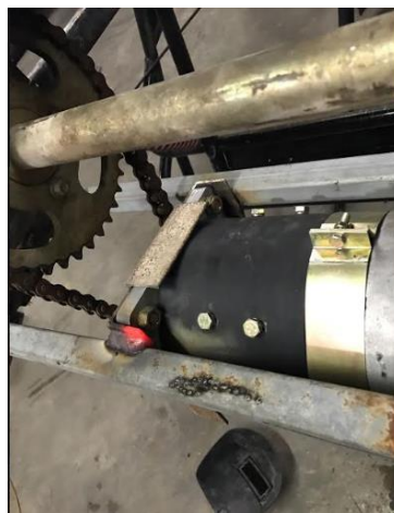
Figure 4.5: Mounting of DC motor in the car
