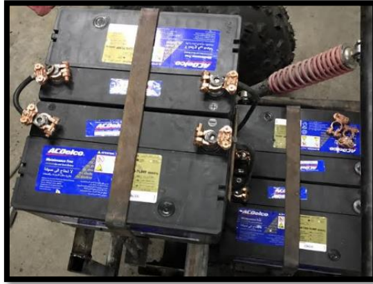
Figure 4.2: Series Connection for Batteries
