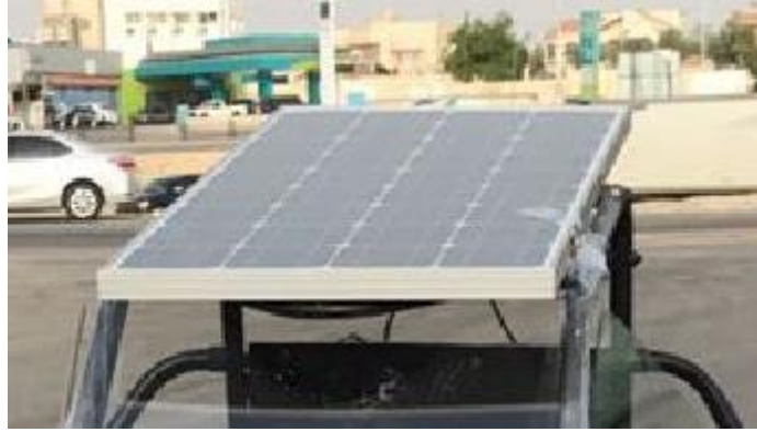
Figure 4.4: Mounting of Solar Panel on the Car
