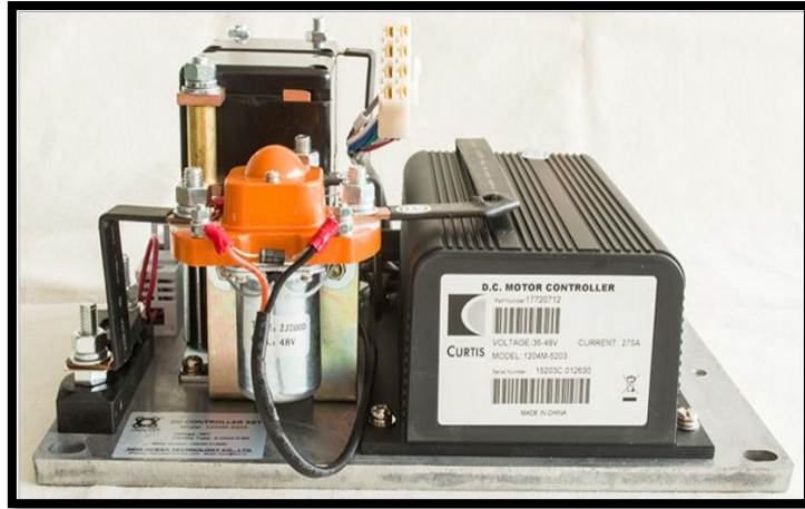
Figure 3.4: CURTIS DC Series Motor Controller Assemblage
