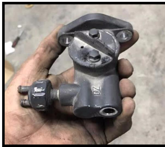
. Figure 4.6: Malfunctioned Brake Master Cylinder
