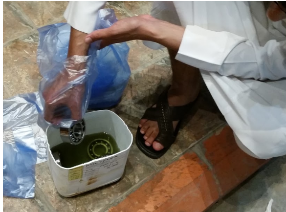
Figure 4.1 - Soaking bearings in bucket with solvent
