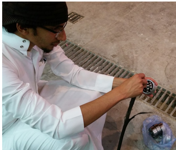
Figure 4.2 - Drying the bearings with compressed air
