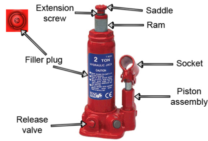
Figure 3.8 – Hydraulic Jack
