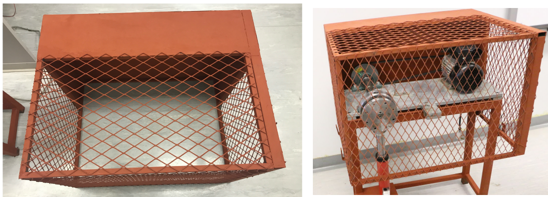
Figure 3.37 - Safety cage (left), Safety cage placed on test rig (right)
