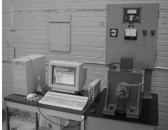
Figure 2.20 - Bearing condition diagnosis and prognosis experimental setup
