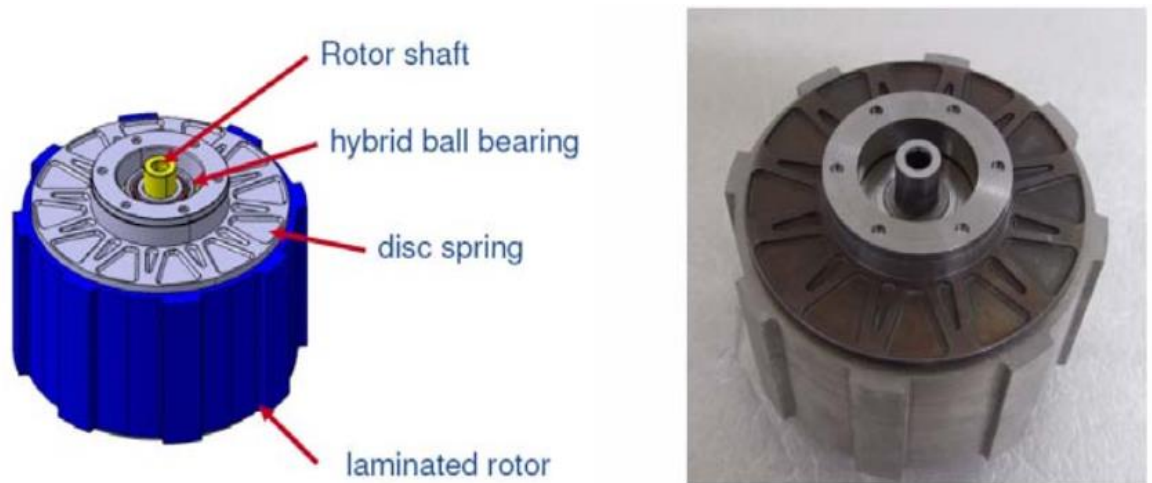
Figure 3. Flywheel rotor of storage subunit [3]
