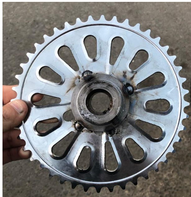
Figure 3.17 Sprocket welded to the key
