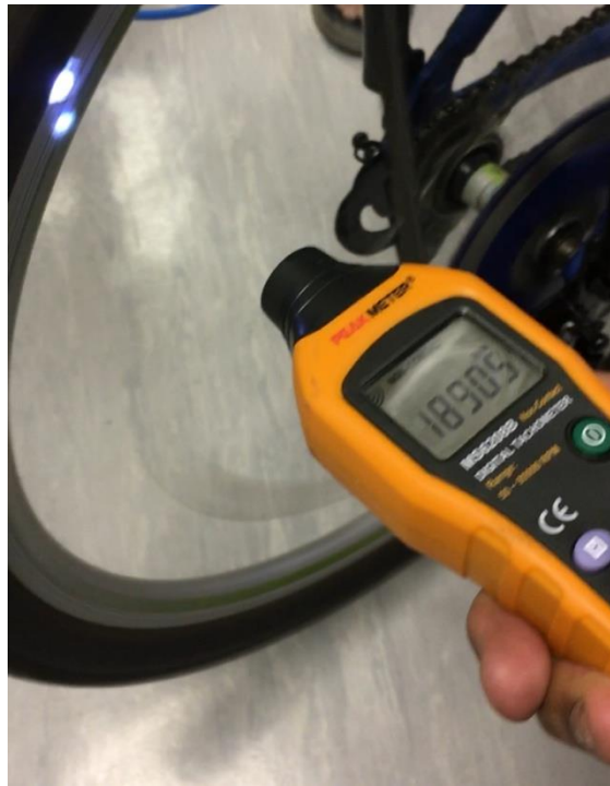
Figure 4.5 rpm of wheel with engine running with 5 bar
