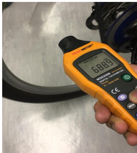
Figure 4.4 rpm of wheel without engine running
