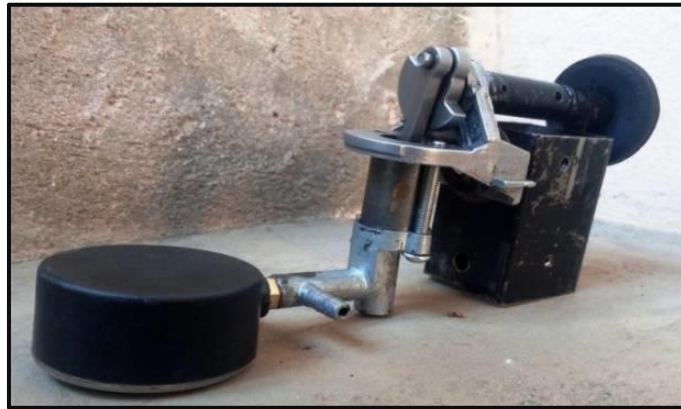
Figure 2.12 Compressor coupler assembly [21]
