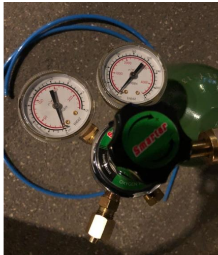
Figure 3.11 Regulator connected to Pneumatic Hose
