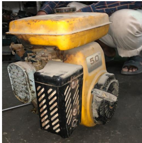
Figure 3.6 Robin EY-20 Generator before disassembly
