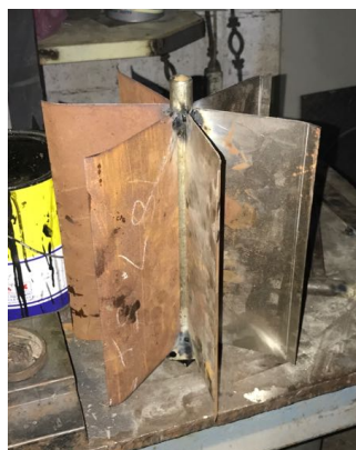
Figure 3.3: The blades of the fan welded to the shaft
