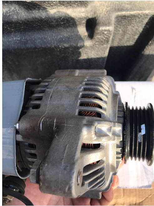
Figure 4.2: pulley of the alternator
