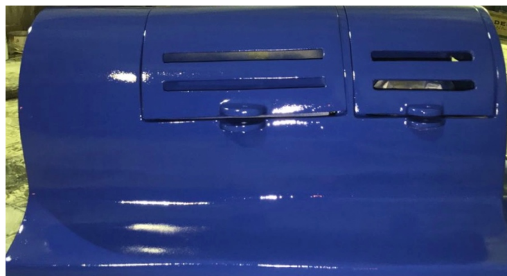
Figure 3.8: Back of the system after fiberglass
