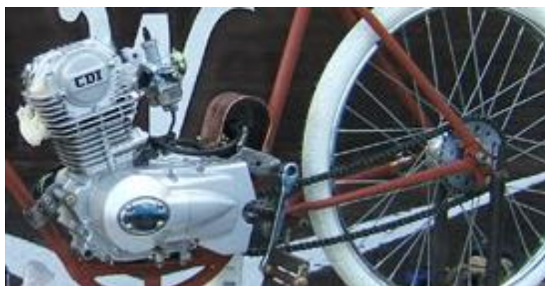
Figure 2.10: The final fabrication of the motor in the bicycle [10]
