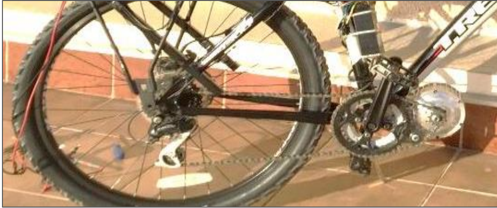
Figure 2.7: A motor connected to the chain wheel [8]
