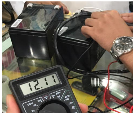
Figure 4.1: A Multimeter to measure the voltage
