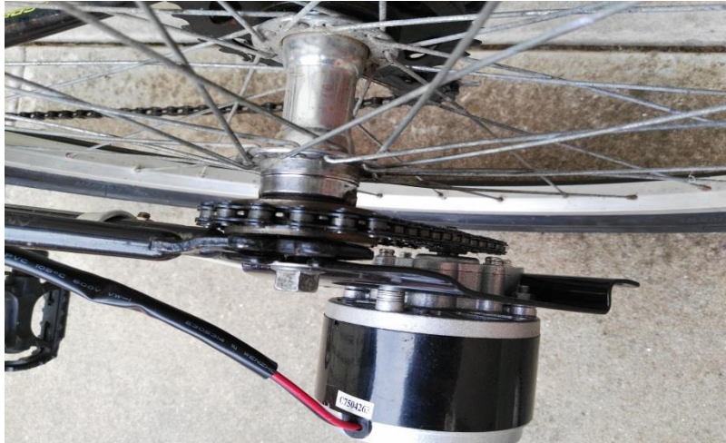
Figure 2.9: The motor connected the hub by a chain [9]
