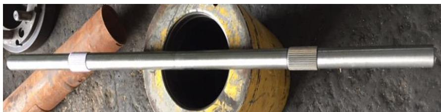
Figure 3.2: Shaft used for our dynamometer
