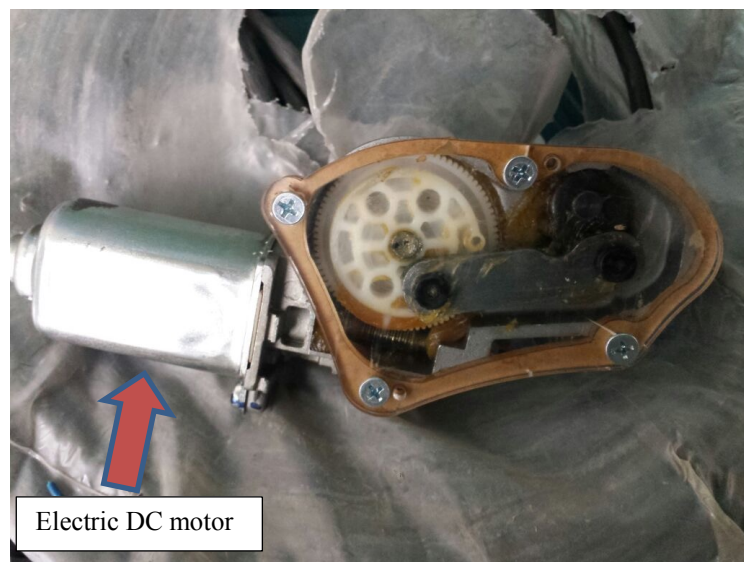
Figure 3.4 (input power system)
