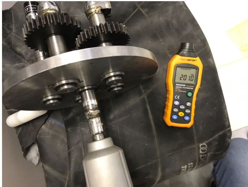
Figure 4.2: Calculation of speed using a tachometer
