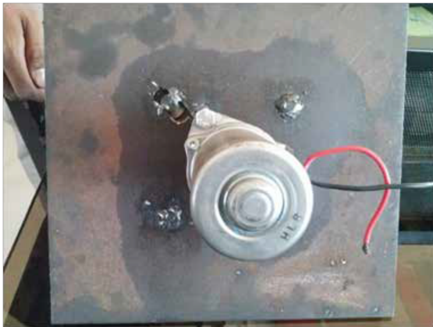
Figure 2.7: In the back view, the motor arrangement can be seen. The motor is connected to the shaft which is connected to the primary gear.
