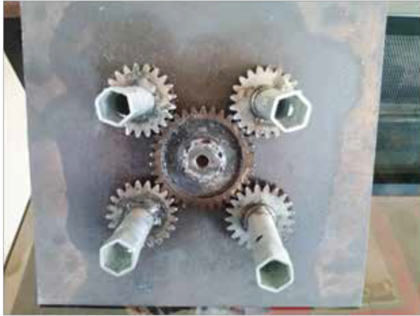
Figure 2.6: In the front view, the gear arrangement and the tool arrangement can be viewed.
