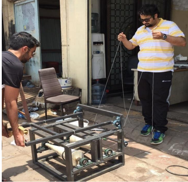
Figure 24 (Testing Driven Cone & Weight Bar)
