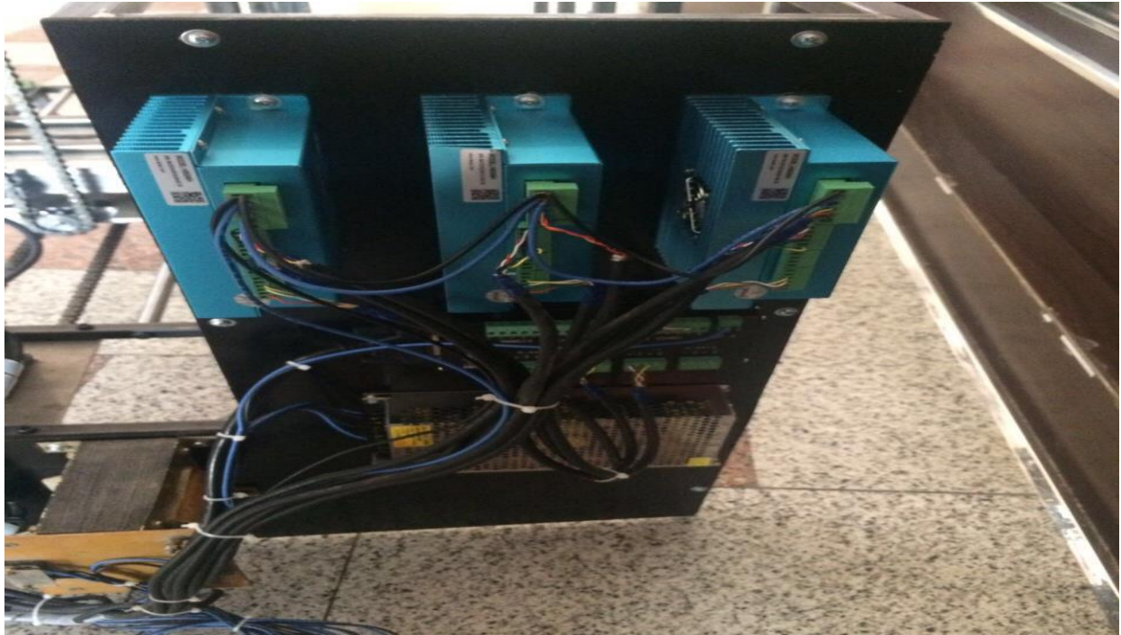
Figure (4.2): Three controllers
