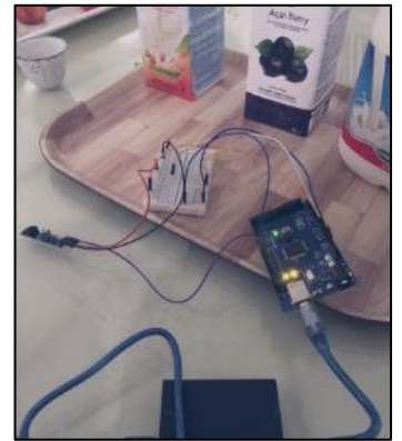
Figure 1.4: Implementation of the IR sensor for the juice and milk.
