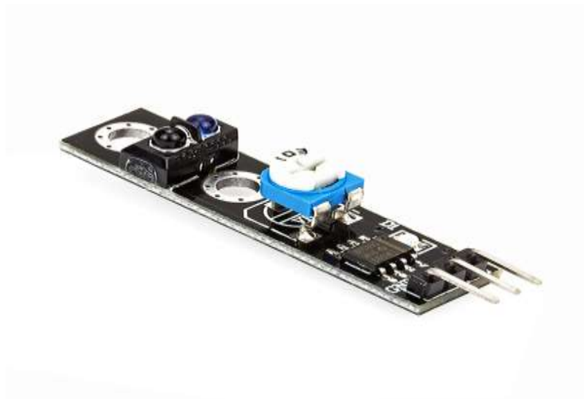
Figure 17: IR line following sensor used in subsystem 3 of the restaurant service system (RSS) project.
