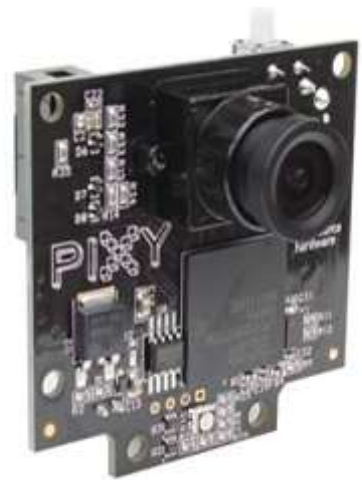
Figure 25: Pixy cam used in the restaurant service system (RSS) project.
