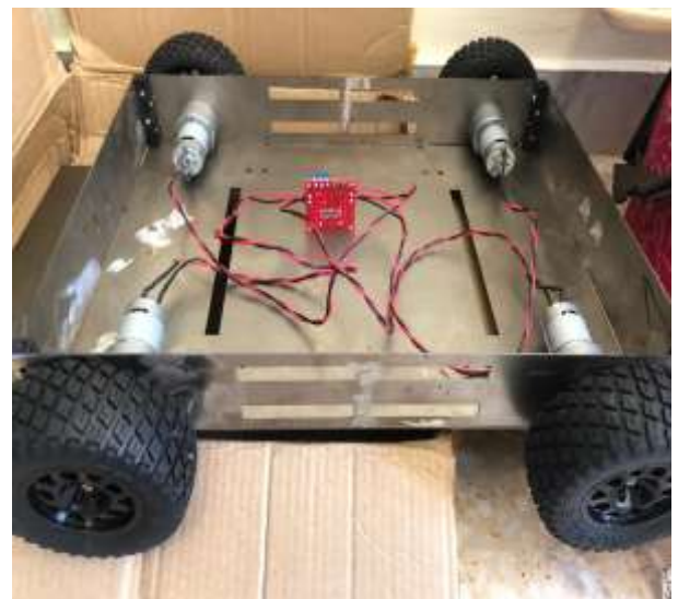
Figure 22: New chassis of the restaurant service system (RSS).
