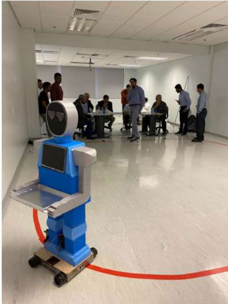
Figure 34: Final prototype of the restaurant service system (RSS) while functioning to go to a designated table.
