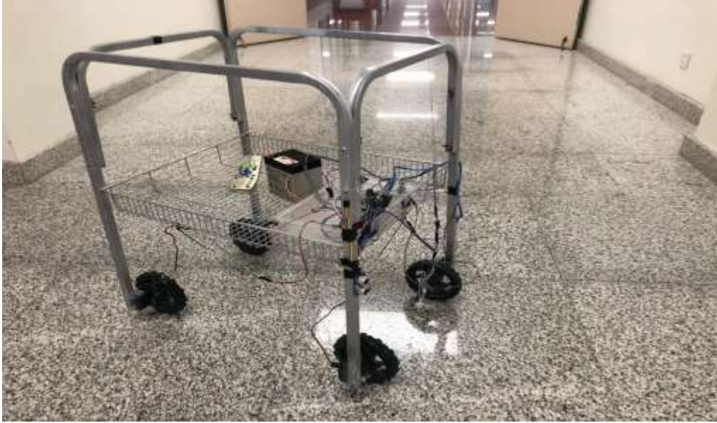
Figure 2: Old chassis of the restaurant service system (RSS).
