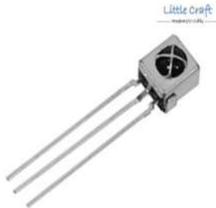
Figure 13: IR receiver used in subsystem 2 of the restaurant service system (RSS) project.
