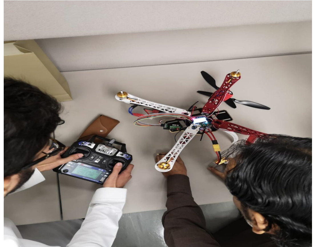
Checking connection of transmitter to receiver and flight controller
