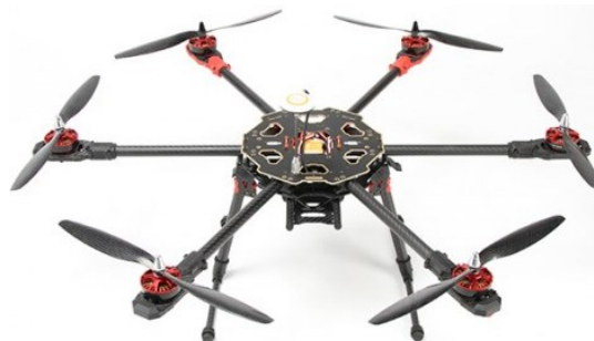
Figure #3.1.1-1: shows the hexa-copter configuration
