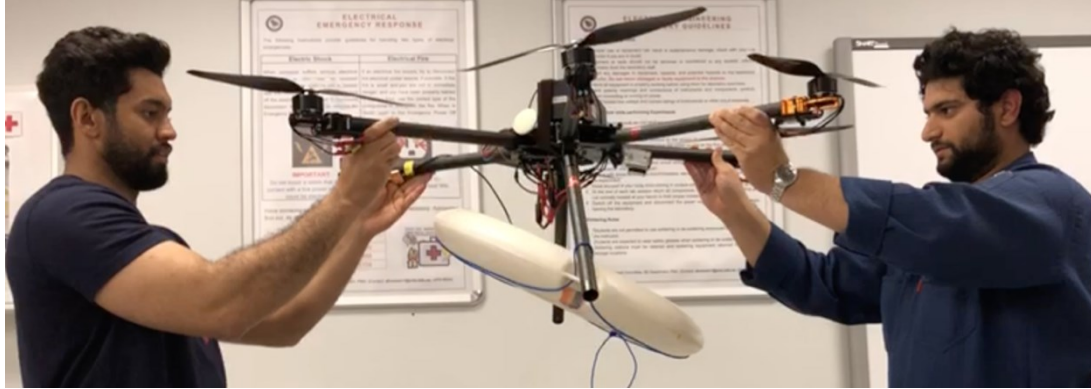
Figure #4.5-1: shows the life ring and life ring holder subsystem while testing
