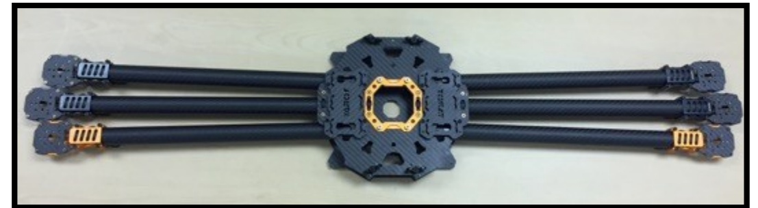
Fixed the completion of the drone frame
