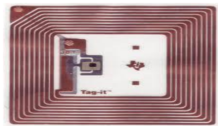
Figure-2.18: RFID Tag Circuit
