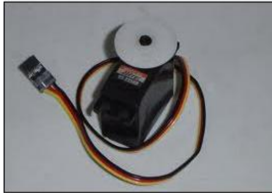
Figure-3.6 : Servo Motor type (HS-5485HB)
