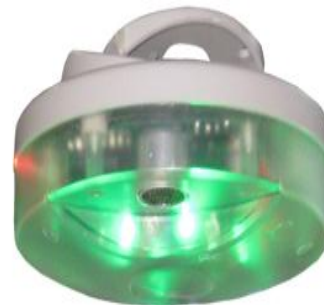
Figure-1.5: OmnyPark OP-511 Ultrasonic Parking Sensor
