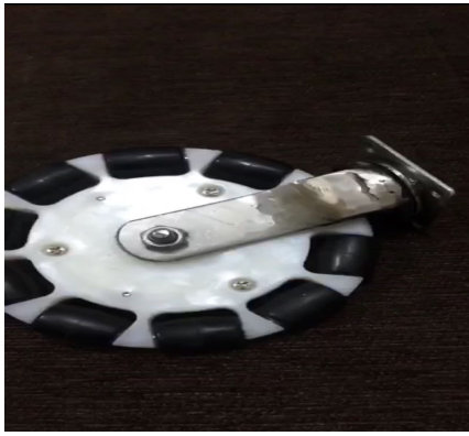
Figure 3.9: The supporting wheel for the front of the vehicle.
