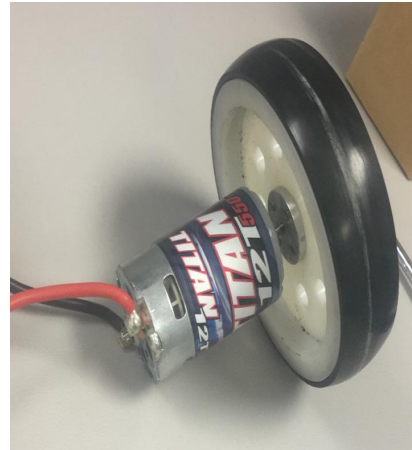
Figure 4.3: Brushed Motor Attached to the wheel
