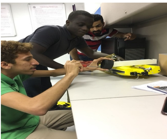
Figure 3.12: Attaching the supporting wheel and the beam
