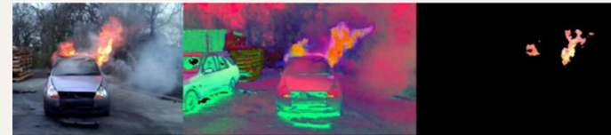
Figure 11: HSV transformed image and fire pixel separated image (image processing)
