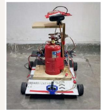
Figure 10: Fire Extinguisher Robot Model
