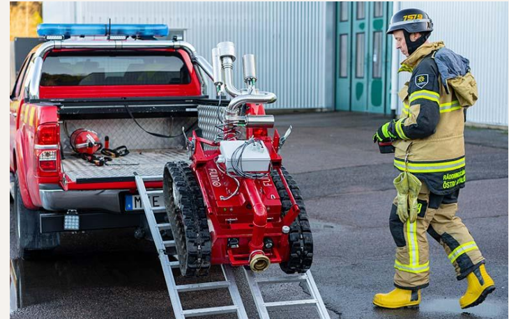
Figure 37: Firefighter utilizing firefighter robot
