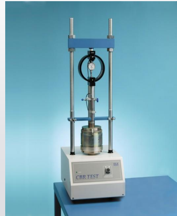
Figure [16]-CBR machine test
