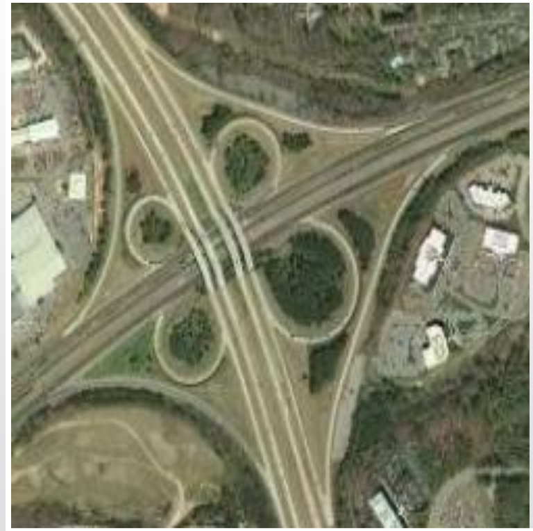
Figure [20]-Grade separation intersection
